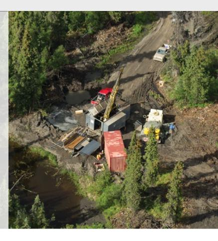
We have three drills running 24/7 for this season's 10,000-meter drill program. The data we collect from the drill cores will help us better understand the grade of the Selwyn Project deposit, the strength of the rock, water flow for the potential pits and the surrounding soil compositions. We'll use the information to complete our Prefeasibility Study (PFS) and Tailing Storage Facility (TSF) studies.
