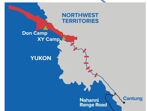
Completed upgrades to the Howard's Pass Access Road in 2014: eight new bridges and road reconstruction to allow all-season access.
